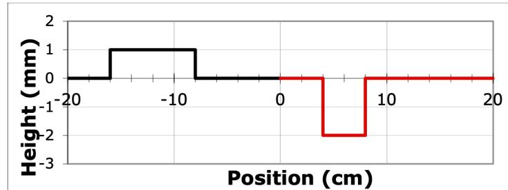
Figure: A point in time of the graph of a square wave after reflecting and transmitting at  $x = 0$ .
